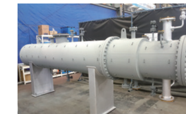
LP Feed Water Heater
