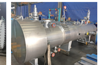
HP Feed Water Heater
